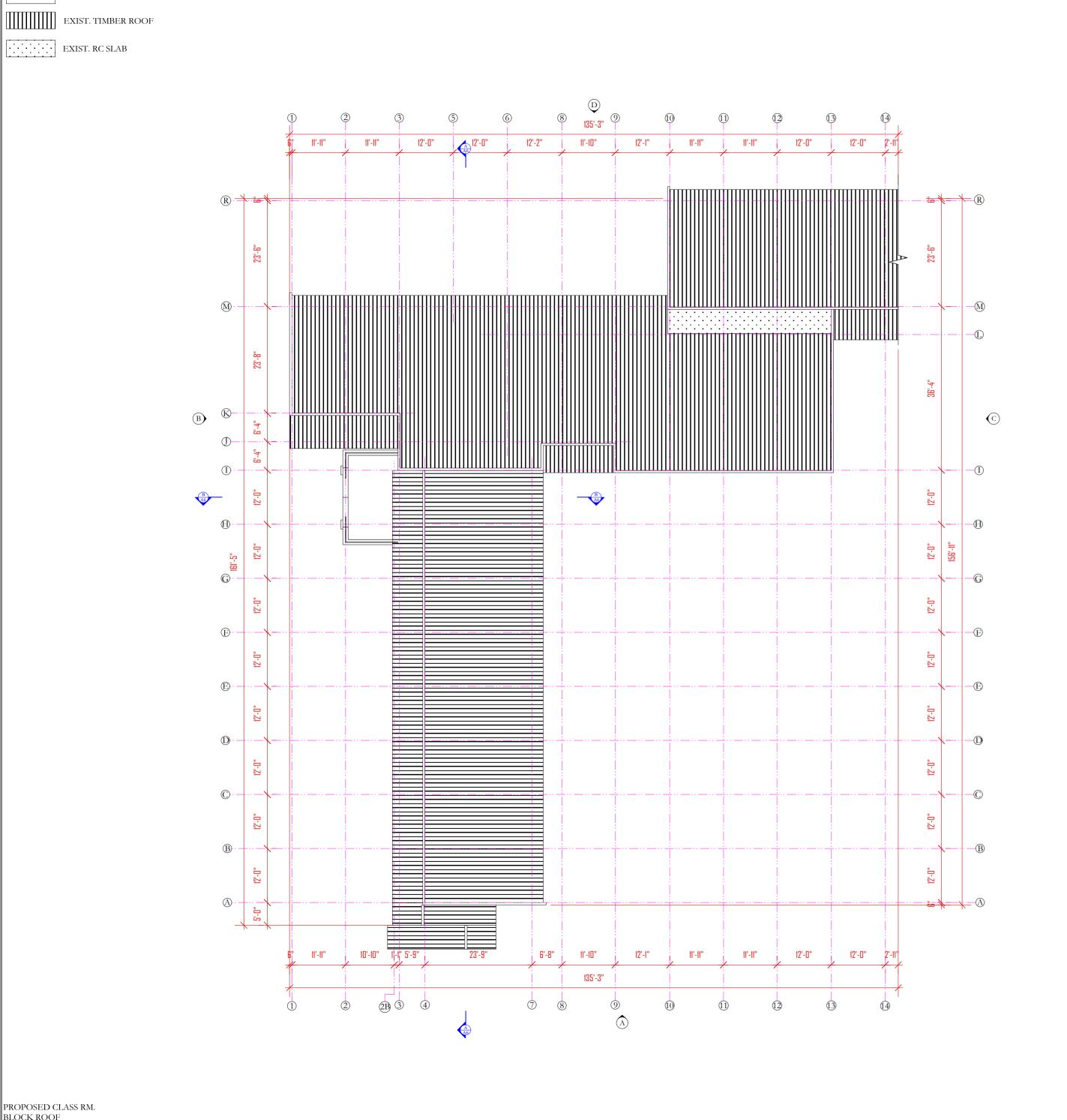
. THESE DRAWINGS ARE TO BE READ INCOJUNCTION WITH ALL STRUCTURAL AND SERVICES ENGINEERS' DRAWINGS. . IF YOU ARE IN DOUBT PLEASE ASK. . ALL EXTERIOR DOORS SHALL BE FITTED W/ S/S SADDLES . ALL LOCKS SHALL BE MASTER & SUB MASTER KEYED . ALL EXTERIOR DOORS & WINDOWS SHALL WITHSTAND 150MPH WIND MINIMUM GLAZING SHALL BE IMPACT GLASS 7. ELITE ARCHITECTURAL IRONMONGERY OR EQUAL & APPROVED, 3 HINGES PER DOOR, 2 FALLING HINGES PER TOILET DOOR REVISIONS
